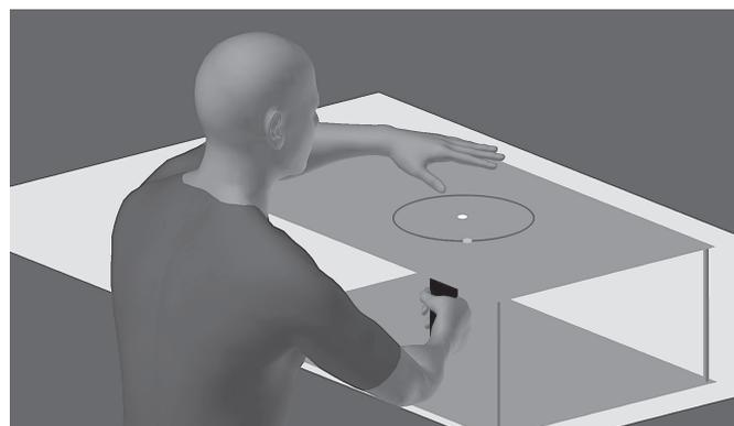
Fig. 1. Experimental setup for both experiments. The subject holds a digitizing pen in his right hand, which is covered by the touch screen. The left hand is used to tap the touch screen on the blue ring to report the aiming location before each trial. After the subject taps on the screen, the blue aiming ring disappears and the orange target turns green.
